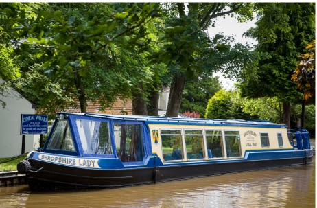
large deck, reached by ramp or lift, an alternative hydraulic joystick steering and cctv screen, an open galley and saloon with comfortable seating and a recliner, huge windows and skylights for all-round visibility. She has also been fitted with a powerful bow-thruster to ensure no bumps when the boat is turning.
